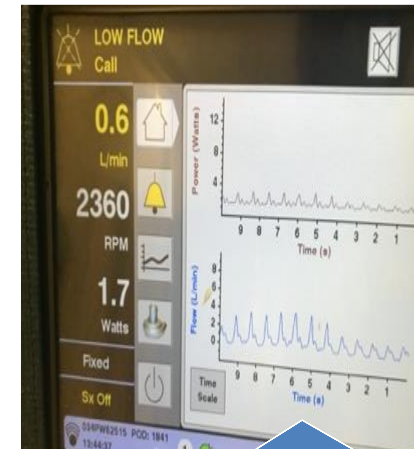
a. Left ventricular assist device (Heartware HVAD Medtronic) waveform during balloon occlusion of the outflow graft resulting in further reduction in waveform pulsatility and flow.
